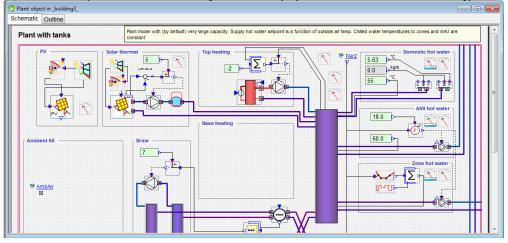
Screen capture of sample system, involving solar thermal and PV
