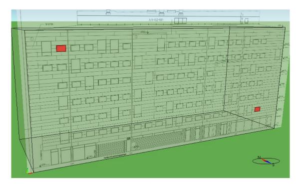
9. Select the two windows with the mouse while holding down the shift-key. Place the cursor on top of one of the windows, right-click and choose Grid from the menu. The Specify grid parameters dialog is opened with X min, X max, Y min and Y max taken from the two existing windows. X step and Y step are calculated from these and from the number of rows and columns. Change the number of rows to 6.
