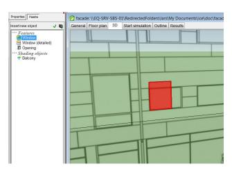
8. Move the window you added to the top left of the façade by selecting it in the 3D view and dragging it while holding down the ctrl-key. Add a second window by dragging a window of the new type from the palette. Place it in the lower right of the façade.
