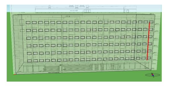
Drag the grid line to the left while holding down the ctrl-key. Align the column with the windows to the left.
